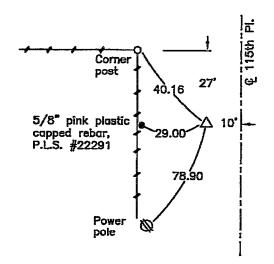
NOTE: ALL TIES ARE PLUMB MEASUREMENTS TO ORANGE SURVEY MARKER UNLESS NOTED.
