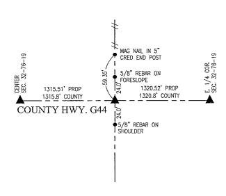
OCTOBER 2018 - PLS 14416 ESTABLISHED CORNER ON LINE AND PROPORTIONATE DISTANCE BETWEEN CENTER AND E. 1/4 CORNER OF SECTION 32.
