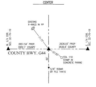
OCTOBER 2018 - PLS 14416 ESTABLISHED CORNER ON LINE AND PROPORTIONATE DISTANCE BETWEEN W. 1/4 CORNER AND E. 1/4 CORNER OF SECTION 32. PROPORTIONATE DISTANCE BASED ON COUNTY HIGHWAY R.O.W. PLAT IN MISC. REC. 6U PAGE 209. SET MAG NAIL IN CONCRETE PAVING 0.3' NORTH OF CL JOINT.
