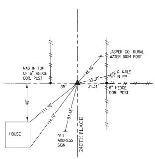
OCT. 10, 1970 - PLS 6708 COUNTY REFERENCE TIES NOTE IRON PIN OVER WPA CONCRETE MONUMENT. DUG HOLE BUT COULD NOT FIND PIPE OR CM. REFERENCE TIES CROSSED WELL SO USED FOR CORNER
