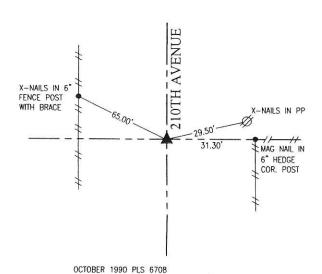
FOUND WPA CONCRETE MONUMENT 18" DEEP IN LINE WITH FENCE EAST AND SLIGHTLY EAST OF CENTER OF ROAD. SET 5/8" X 30" REBAR ON NORTH SIDE OF C.M. AND 5/8" X 10" REBAR 4" DEEP ABOVE C.M. SET 60D NAIL AND BLUE TOP AT SURFACE.
