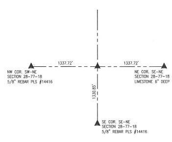
DECEMBER 4, 2020 SET  $5/8^\circ$  X 30° REBAR WITH CAP #14416 ON LINE AND MIDWAY BETWEEN NW CORNER SW-NE AND NE CORNER SE-NE.
